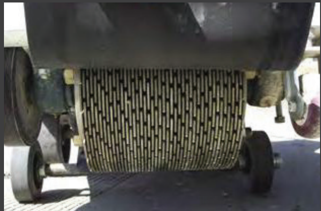
Uses 12" diameter blades on a 10" or 16" grinding head with specifications that can be custom fit to your application
