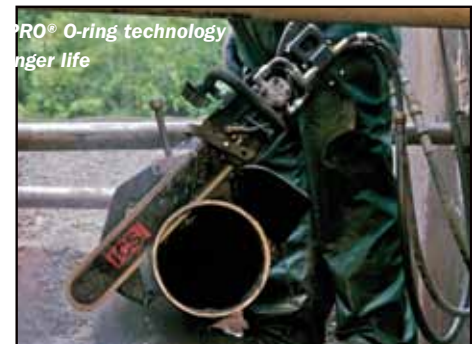
Hydraulic Saw is completely submersible
