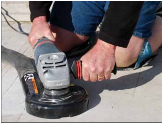
The IXL full shroud is designed for open areas.
