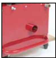
Vacuum port helps in dust control
