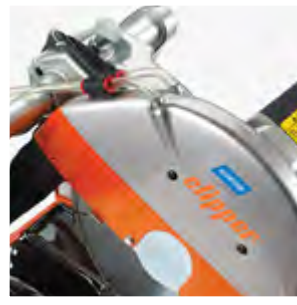
Pivoting Locking Head Plunge/step cutting and jam cutting (all the way down).
